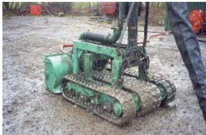
Double Track Systems for Clay lining
