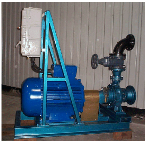
Pump for one Tanksweep 250m 3 /h at 10bar 132kw
